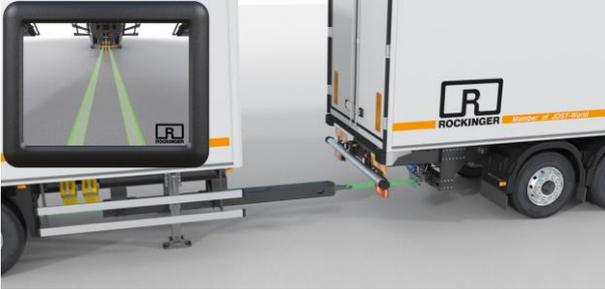
**Command Steer Axle JOST CSA with electronic steering system TRIDEC EF-S:**
